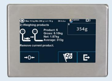
The operator is first instructed to weigh a frozen box full of product and then proceeds to weigh each and every defrosted product contained in the box. This results in a detailed report dealing with the frozen gross weight, and the weight of each product.
